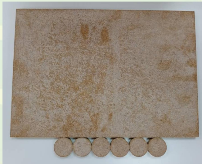
Figure 1. Photograph of 'NEBAR WHITE GASKET; Brand: James Walker; Type of product: GASKET; Size: 1200 mm x 1200 mm; Thickness: 6.4 mm' Test Specimens
